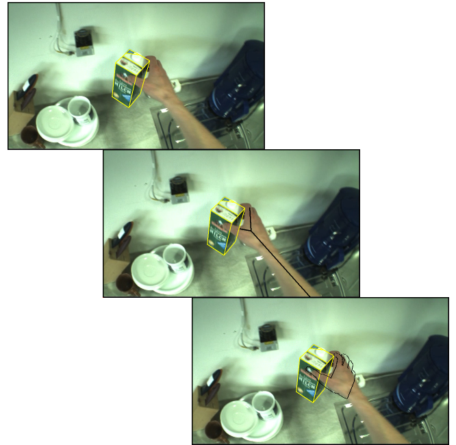
Fig. 8. Processing steps in fitting object and hand models to the images from the head mounted camera: 1) matched object model; 2) matched 2D hand model; 3) matched 3D hand model.
