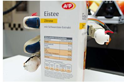
Fig. 4. Three fingertip sensors installed in the DLR/HIT hand (thumb, index and ring fingers).
