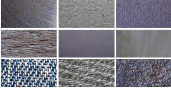
Fig. 15. Macro images of the different material surfaces used in the second classification experiment. From left to right and from top to bottom: (1)metal, (2)table melamine surface, (3)paper, (4)wood, (5)plastic, (6)glass, (7)fabric, (8)napkin paper and (9)cardboard.
