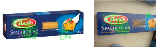
Fig. 7. A sample image found on Google for Barilla (left) and an image taken with a consumer camera as a test case on the right side. Extracted features are visualized with green markers.
