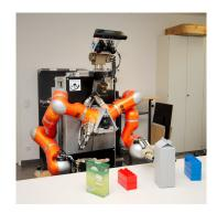
Figure 1. Different objects mostly require different grasping techniques and may not obstruct each other when placing them.
